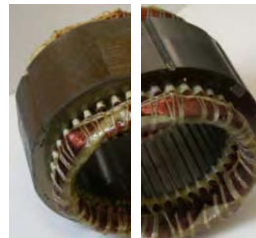
Figure 2: Stator part with semi-closed slots (right) and the novel construction without any slots (left).
