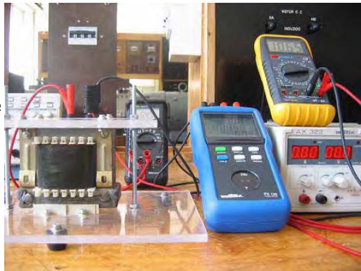
Fig.4 Electromagnet in attracted position and experimental setup for DC supply.
