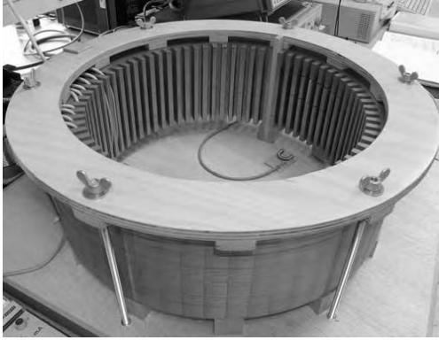
Fig. 1. Test core for investigation of interlamination short-circuits for different positions and strength.
