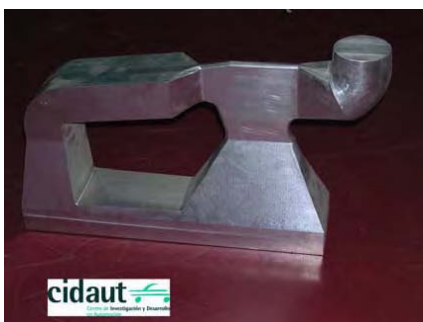
Fig.5 Solid secondary that substitutes the channel carrying molten aluminium.
