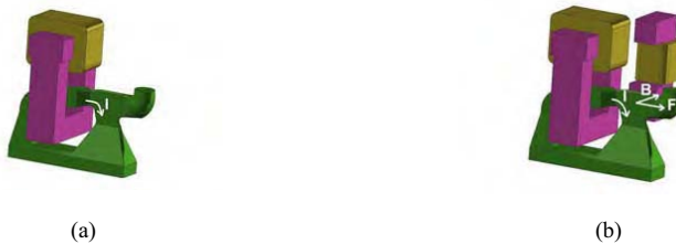
Fig.2 Electromagnetic pump operating principle.
