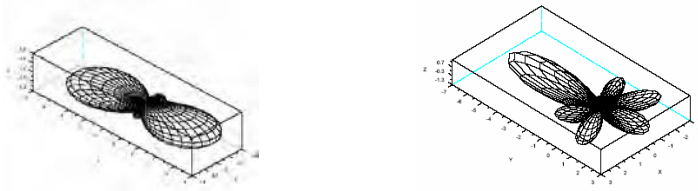
Fig.1 Radiation pattern of a dipole antenna in the presence of a human head at 900 (left) and 1800 (right) Mhz – Non uniform (4-tissues) model.
