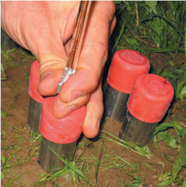
Figure 6.8 Field-chamber approach for determining in situ biogeochemical activity. Shown is a cluster of open-ended stainless steel cylinders inserted into the soil surface. After being capped with red rubber septa, the cylinders allow changes in the concentration of head-space gases to be monitored over time. The gas-sampling syringe (shown) delivers the sampled gas to a gas chromatograph for analysis. The chamber pictured here (and larger ones, sometimes fashioned from plexiglass) is typically installed temporarily over soil or water habitats. Large chambers may be fitted with an internal battery-operated fan to insure uniform mixing of gases (e.g., \text{CO}_2 , \text{N}_2\text{O} , and \text{CH}_4 ). (From J. Yagi, Cornell University, with permission.)
