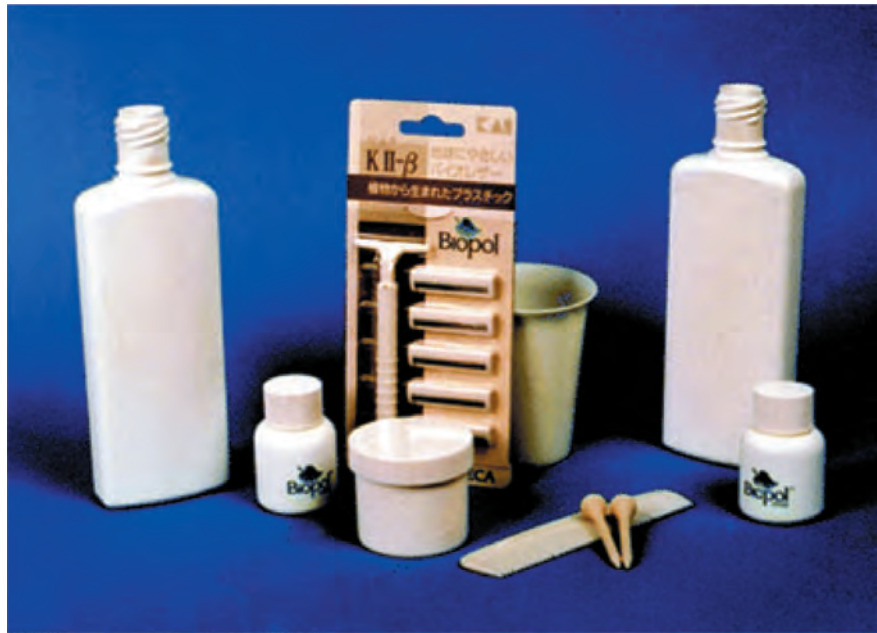
Figure 8.25 Commercially manufactured, biodegradable, molded plastic containers created from microbial polyesters. (Reprinted with permission from Lenz, R.W. and R.H. Marchessault. 2005. Bacterial polyesters: biosynthesis, biodegradable plastics and biotechnology. BioMacromolecules 6:1–8. Copyright 2005, American Chemical Society.)
