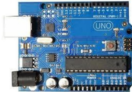
Figure 9.7: Arduino UNO board.
