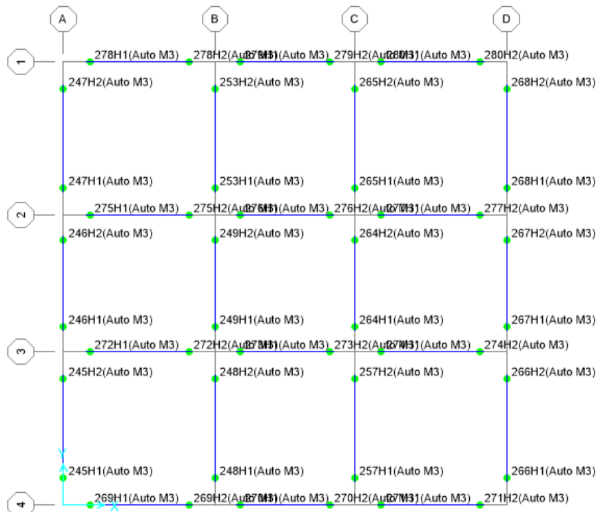
Figure 4.18 Position of Hinge 275H1 at grid 2 & A horizontal & vertical respectively.at 5th floor
