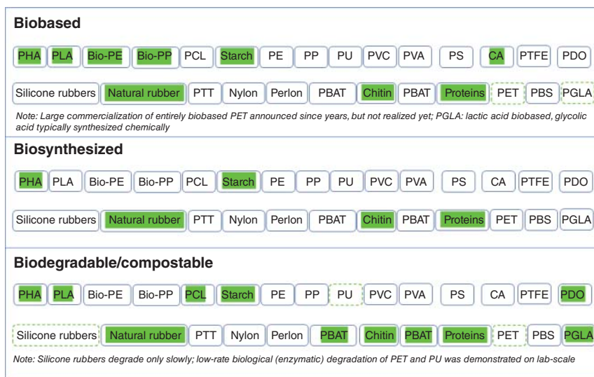
Figure 1.7 Classification of diverse polymers. Polymers marked in green meet the criteria “biobased,” “biosynthesized,” or “biodegradable/compostable.” PHA: polyhydroxyalkanoates; PLA: poly(lactic acid); Bio-PE: biobased poly(ethylene); Bio-PP: biobased poly(propylene); PCL: poly( \epsilon -caprolactone); PU: poly(urethane); PVC: poly(vinyl chloride); PVA: poly(vinyl alcohol); PS: poly(styrene); CA: cellulose acetate; PTFE: poly(tetrafluoroethylene) (Teflon®); PDO: poly(dioxanone); PTT: poly(trimethylene terephthalate); PBAT: poly(butylene adipate terephthalate) (Ecoflex®); PET: poly(ethylene terephthalate); PBS: poly(butylene succinate); PGLA: poly(glycolic- co -lactic acid). Nota bene : PHA is the only group marked in green in all categories which displays plastic-like properties without the need for special processing techniques and/or additives.
