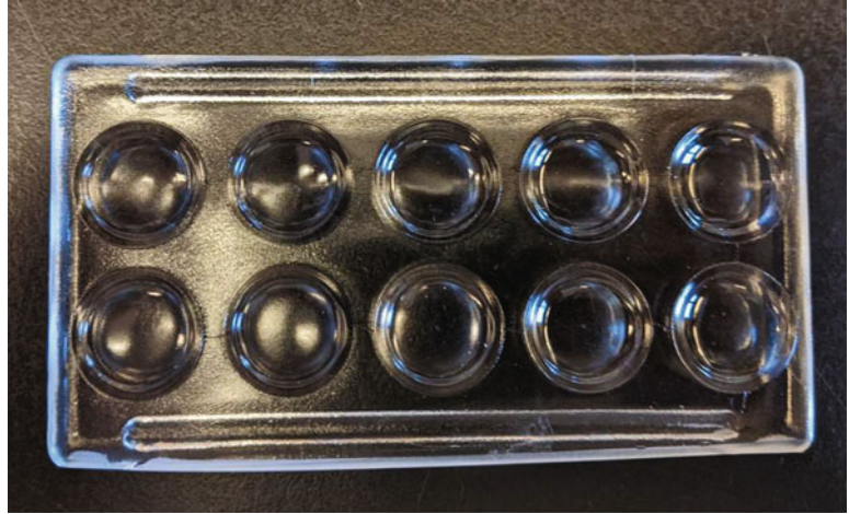
Fig. 4 A 10-well glass plate. This plate can be used to clean the worms and perform the dissection
