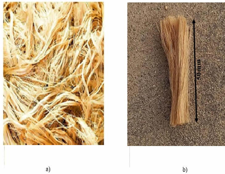
FIGURE 3.2: Jute fibers; a) raw fibers, b) fiber cut length
