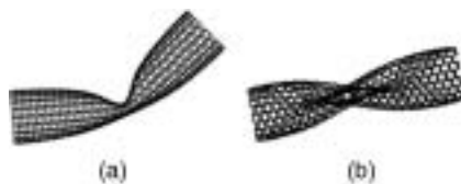
FIGURE 19.9 (a) Buckling of SWCNT under bending load. (b) Buckling of SWCNT under torsional load.
