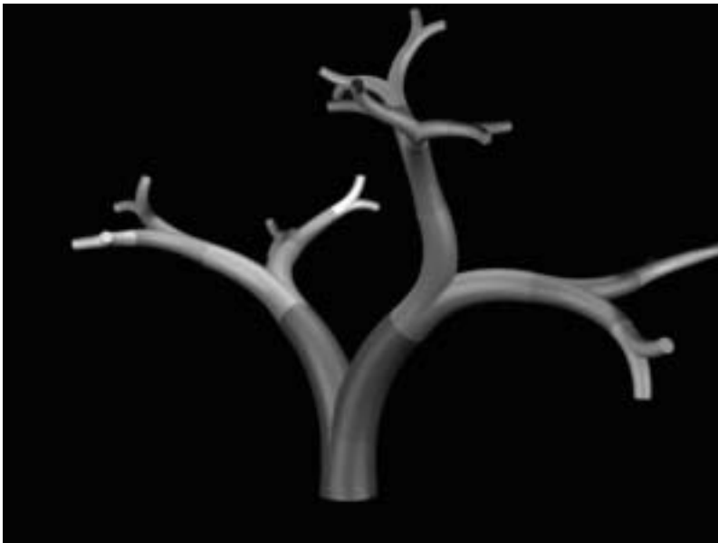
FIGURE 18.9 An illustration of a four-level dendritic neural tree made of 14 symmetric Y-junctions of the type in Figure 18.8 .
