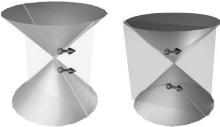
FIGURE 11.12 Lowest conduction sub-band and highest valence sub-band of a metallic tube (left) compared with semiconductor nanotube (right). A nanotube quantization condition makes cut from the cone-shaped bands of graphite. In the case of metallic nanotube, this cross-section passes through the Fermi point and no gap develops between sub-bands. The electron dispersion is linear in longitudinal wave vector. In the case of semiconductor nanotube, the cross-section is shifted away from Fermi point. The carrier dispersion is a hyperbola.
