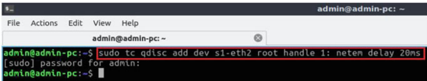
Fig. 108 Adding 20 ms delay to switch S1's s1-eth2 interface
