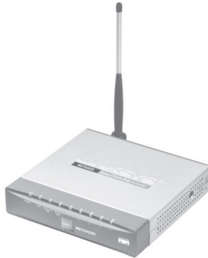
Figure 5-10 A wireless network bridge with a built-in five-port switch
