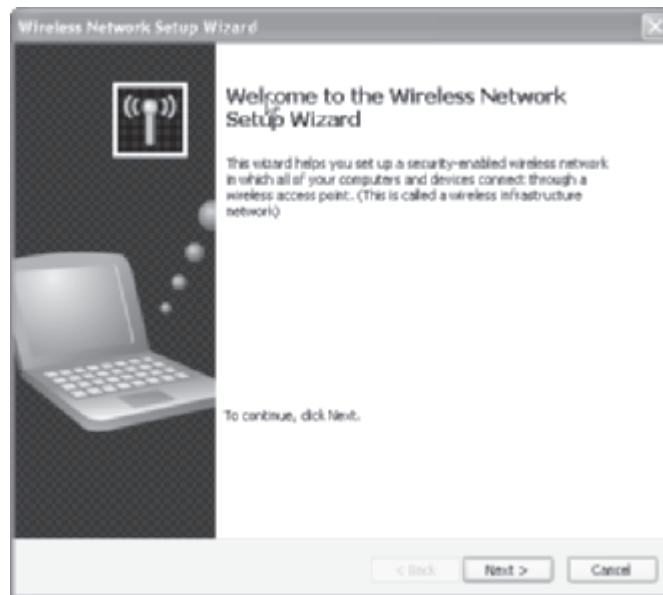
Figure I-11 Run the Windows XP Network Setup Wizard or the Wireless Network Setup Wizard on each PC to create a LAN.
