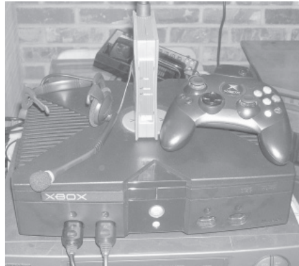
Figure 13-14 An Xbox game console is linked to the home network via a wireless Ethernet bridge (middle top)
