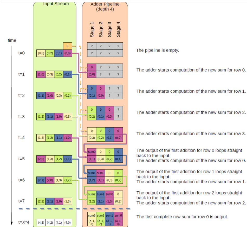
Figure 3. An example of a pipeline for the aggregated sum with different states.
