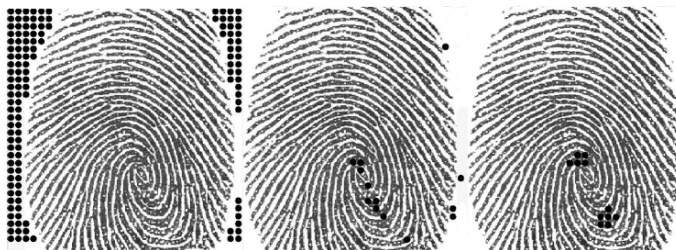
Fig. 18.1 Generated image maps by the MINDTCT algorithm from left to right: low contrast map, low ridge flow map and high curvature map
