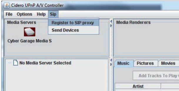
Fig. 4.5 The home A user registers the control point in the SIP proxy
