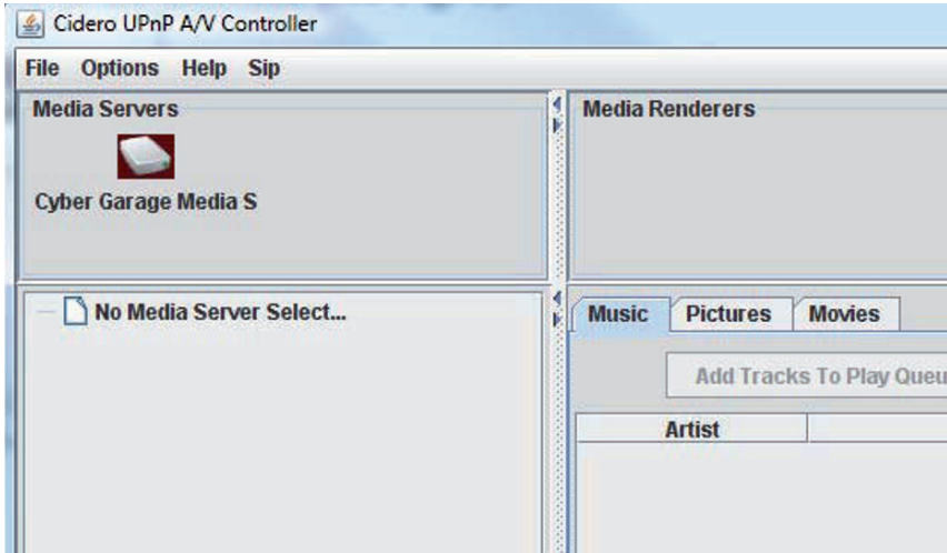
Fig. 4.3 Local detection of UPnP AV devices by the cidero control point at home A
