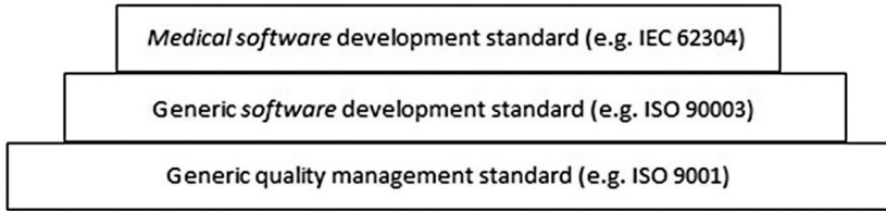
FIGURE 16.2 The standards pyramid showing a foundation general quality management system at the bottom, with more specific standards layered on top.
