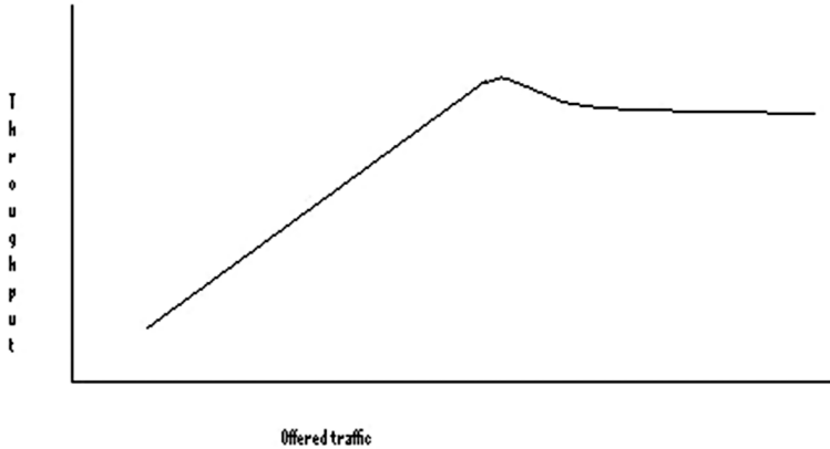
FIGURE 8.17 A generalised throughput verses offered traffic curve showing a deterioration in performance when optimal levels are breached. (Taktak et al. 2019).
