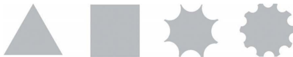
FIGURE 8.5 Top view and side view of four separate rotary control knobs that can be discriminated by touch alone, similar to those tested by Hunt (1953). (© Daniel S. McConnell.)
