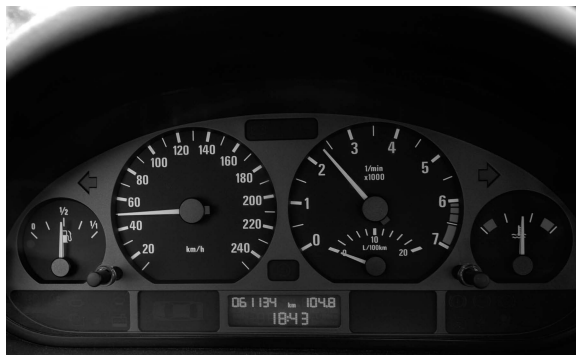
FIGURE 3.8 BMW instrument cluster illustrating the different types of analog, digital, and semicircular displays. (Image available via a CC-BY-SA 3.0 from https://commons.wikimedia.org/wiki/File:BMW_320i_E46_instrument_cluster_during_fuel_cut-off_(aka).jpg .)
