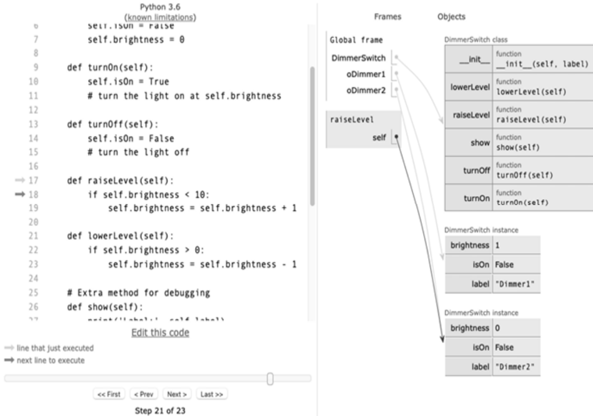
Figure 3-6: The program in Listing 3-3 stopped in call to oDimmer2.raiseLevel()
