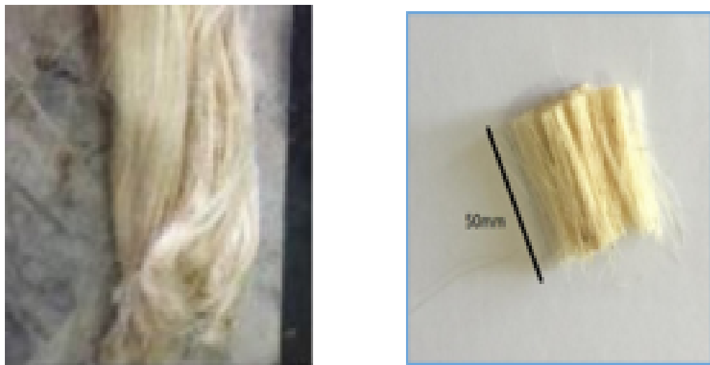
FIGURE 3.1: Jute Fibers: a) Raw Fibers, b) Prepared Fibers
