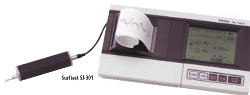
Fig. 3 Device for measurement of surface abrasiveness Mitutoyo SJ 301
