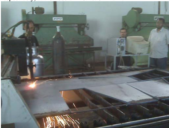
Figure 5. 2D CNC cutting at Mega Forte, Brasília. (Source: photo taken by authors of this paper)
