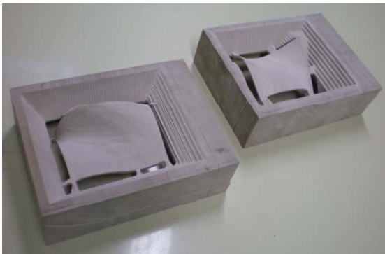
Figure 9. Rapid prototype of the exhibition pavilion of the student Nágila Ramos (Milled in a Roland Modela MDX-40 three-axes milling machine)
