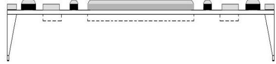
(f) The silicon under the suspended microstructures is removed by anisotropic etching in aqueous \text{KOH} . The movable microstructure can be released to be free-standing.
