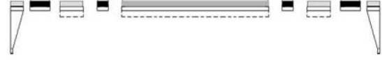
(g) Suspended structures including the mirror plate are released by RIE from the front side of the wafer using the patterned metal film at the step (d) as the masking material.
