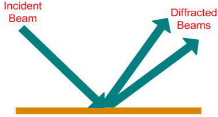
Fig. 4 Multiple Beam steering using Diffraction.
