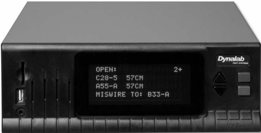
Figure 3.9 The NXPro graphic - the tool that does the point-to-point wire harness checks comparing an input file - DSI from the harness design folks to the received product from the supplier, especially useful on the early prototype parts when deviations may abound with uncertainty of what content is in what harness part number due to the deviations.
