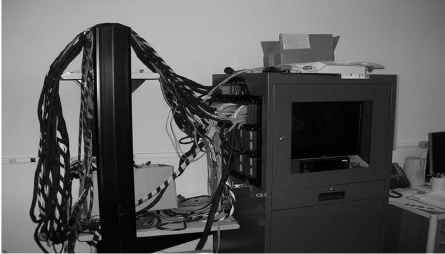
Figure 3.10 Dynalab and cabinet test fixture for automated point-to-point testing.
