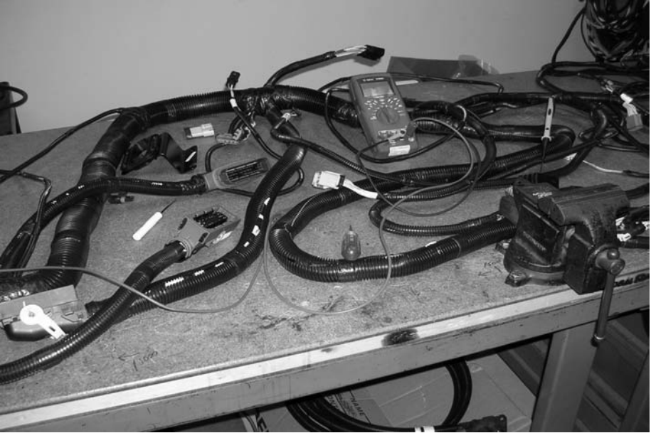
Figure 3.7 Old method of manually testing harness continuity checks.
