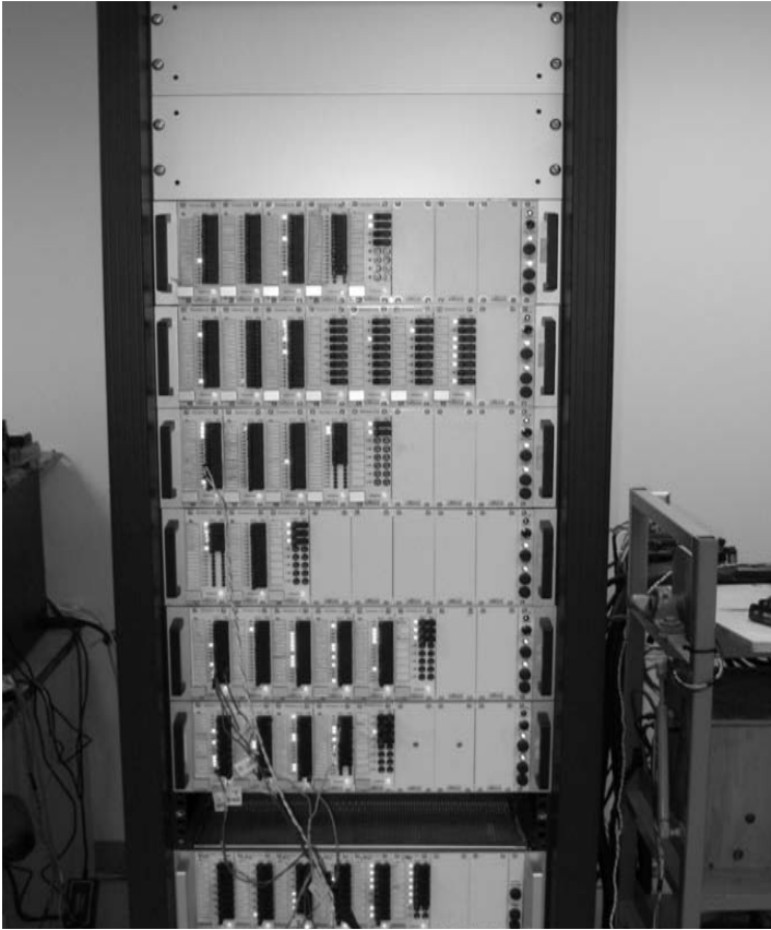
Figure 2.3 A typical test “buck,” with all controllers centralized and powered.
