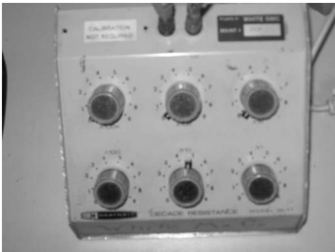
Figure 8.1 Decade box used for testing product response to variation on the resistive inputs of the product.
