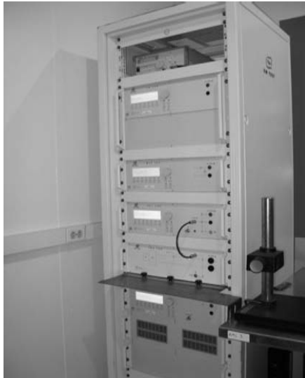
Figure 2.16 Seen is a SAE transient fixture, which replicates EMC bulk current injection and SAE transient simulation/injection.
