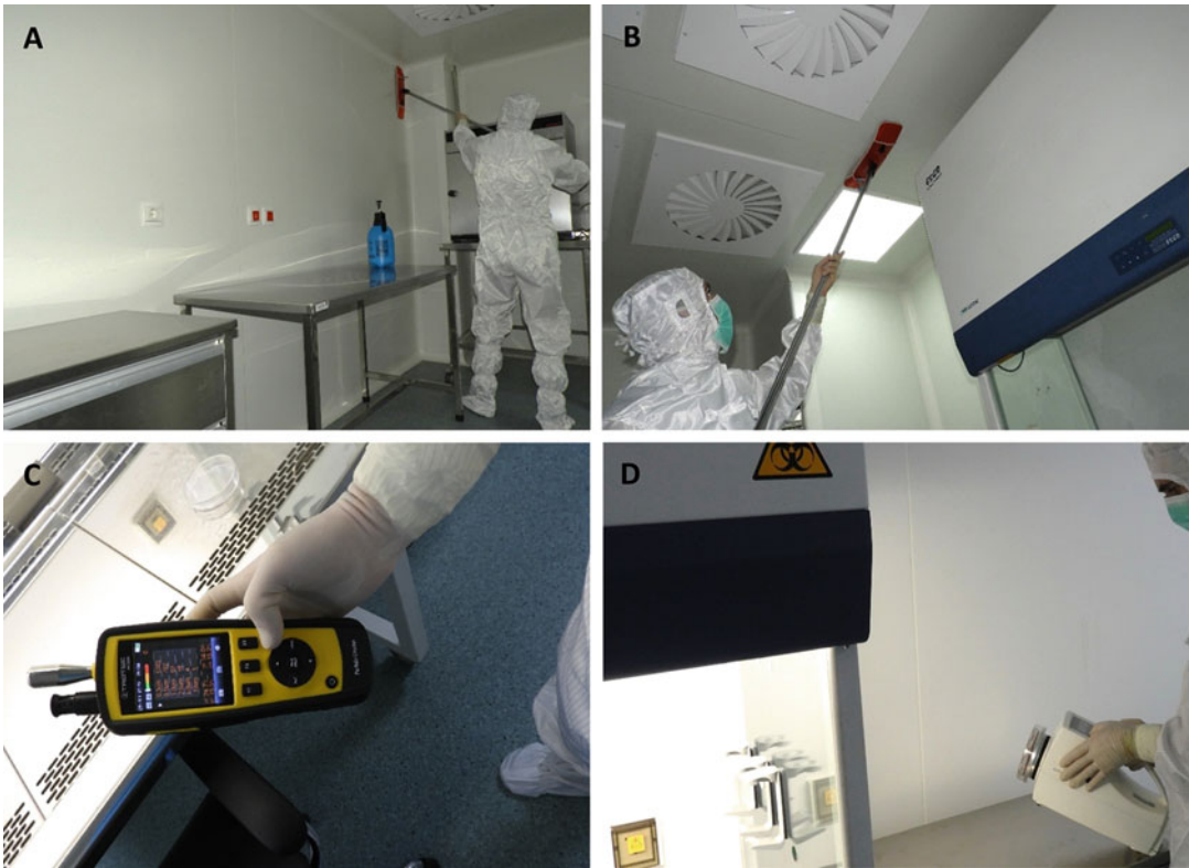
Fig. 1 Clean room maintenance and monitoring. (a, b) Routine maintenance of grade (a) room, (c) nonviable particle counting with laser particle counter, (d) viable particle monitoring with active air sampler
