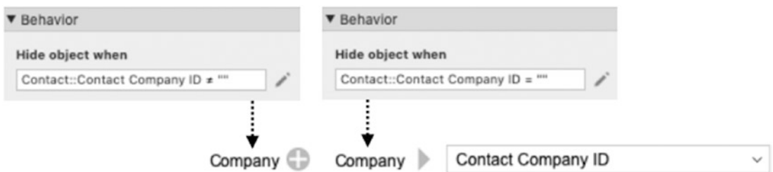
Figure 21-15. A two-segment bar as a field label that always hides one segment.
