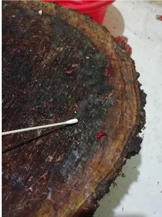
FIGURE 4.2: Sampling from the Surface of Chicken Slaughtering Equipment for Bacteriological Analysis
