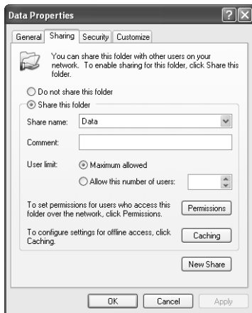
Figure 5-13 After a folder is shared, a New Share button is added that lets you create additional shares.
