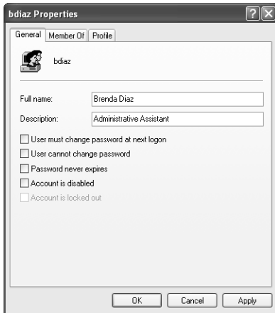
Figure 3-3 Use the General tab of a user account's Properties dialog box to modify basic account properties.
