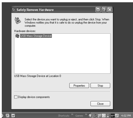
Figure 6-13 Use the Safely Remove Hardware dialog box to stop a device before disconnecting it.
