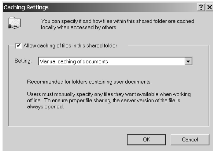
Figure 5-23 On the computer sharing the file, configure the caching (offline file) settings.
