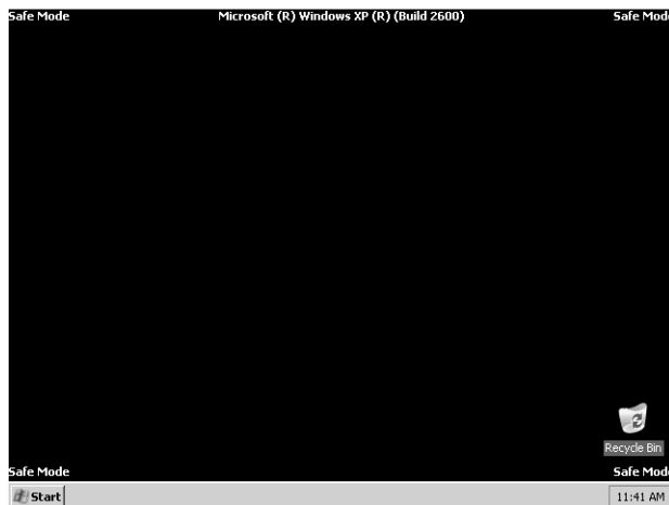
Figure 2-10 Safe mode often allows you to change settings you cannot change in normal mode.
