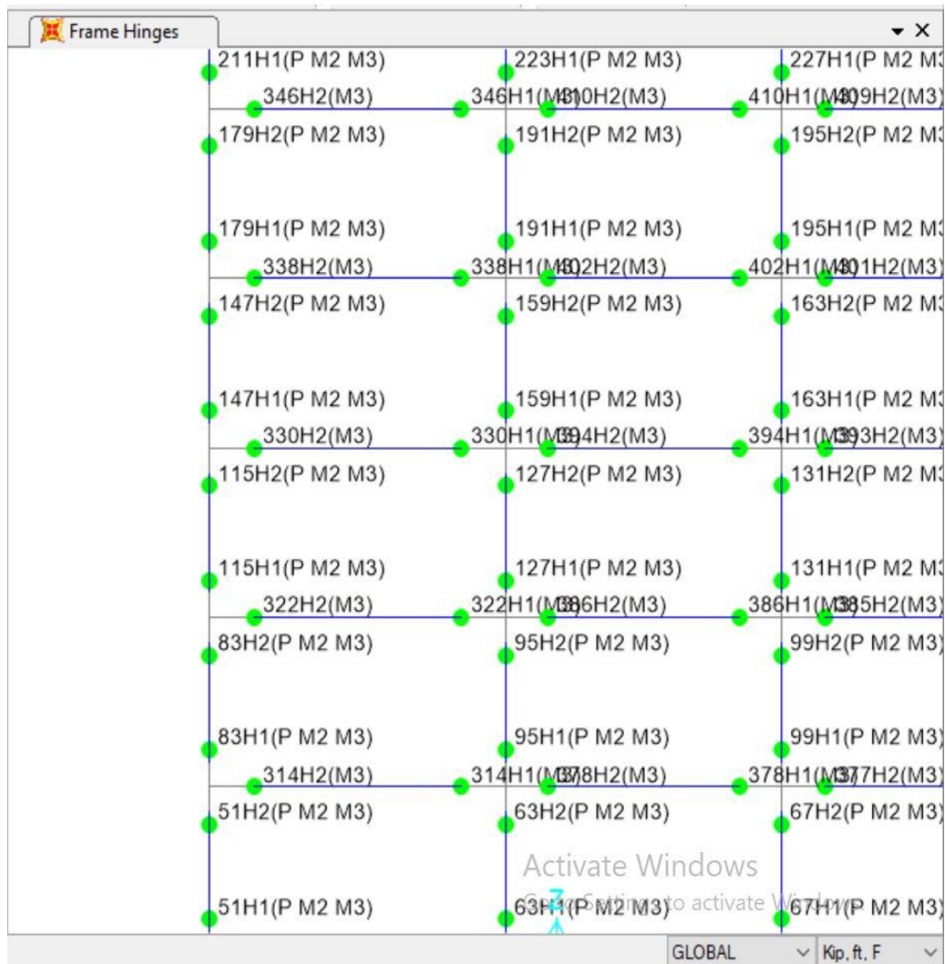
FIGURE 4.14: P-M2-M3 Column Assigned Hinges.
