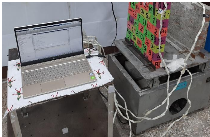
FIGURE 3.6: Shake table instrumentation and testing: a) schematic diagram and b) real test setup
