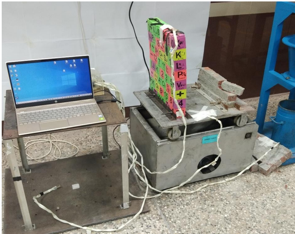
FIGURE 4.3: Failure of unreinforced brick masonry solid wall during testing
