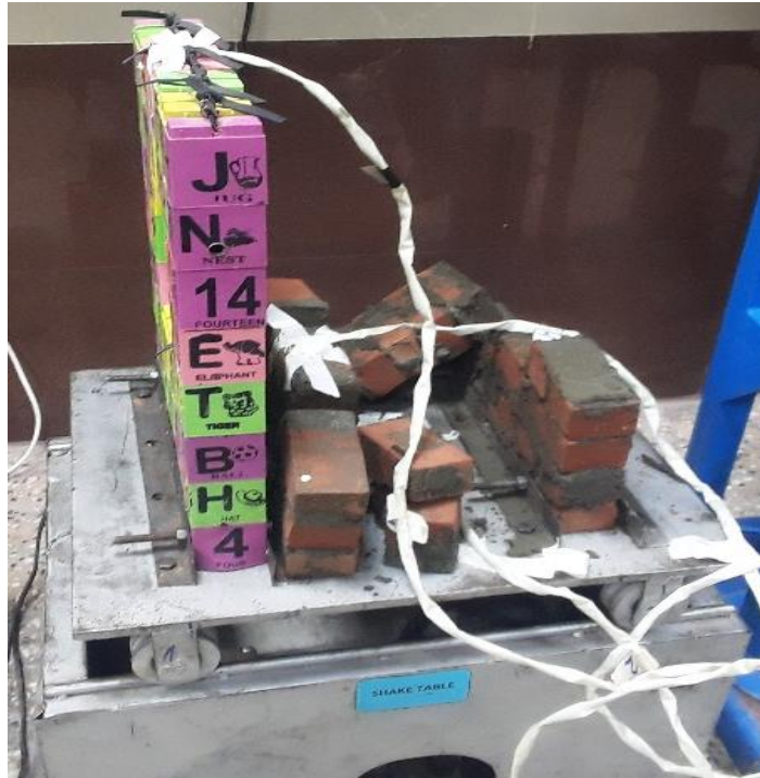
FIGURE 4.4: Failure of unreinforced brick masonry wall with opening during the application of harmonic loading
