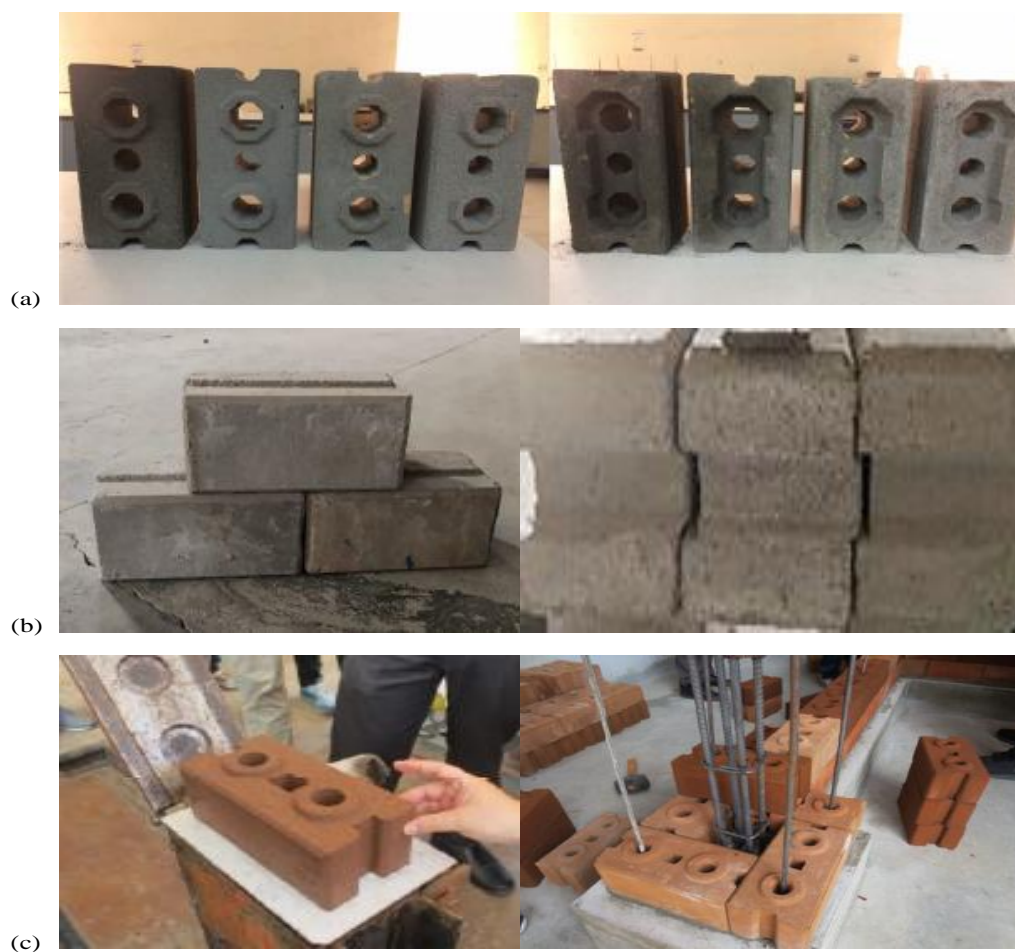
FIGURE 2.7: Various interlocking patterns/techniques for blocks; (a) eco-friendly interlocking block including holes and shapes [27], (b) sliding interlocking block [28], (c) interlocking block including holes to provide steel reinforcement [29]
