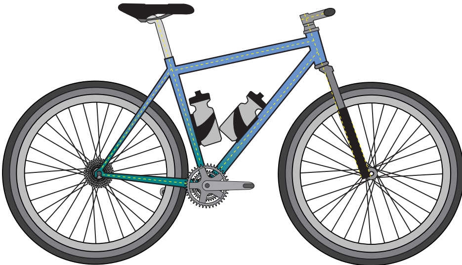
Figure 6.2 Beefy, straight-bar, front-suspension, fat-tired mountain bike
