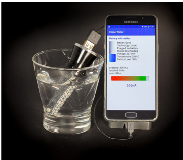
Figure 18.2 Small-scale BDD electrode. The electrode is powered by a mobile phone via USB for the disinfection of potable water (Source: kindly provided by R. Borchardt, Erlangen).
