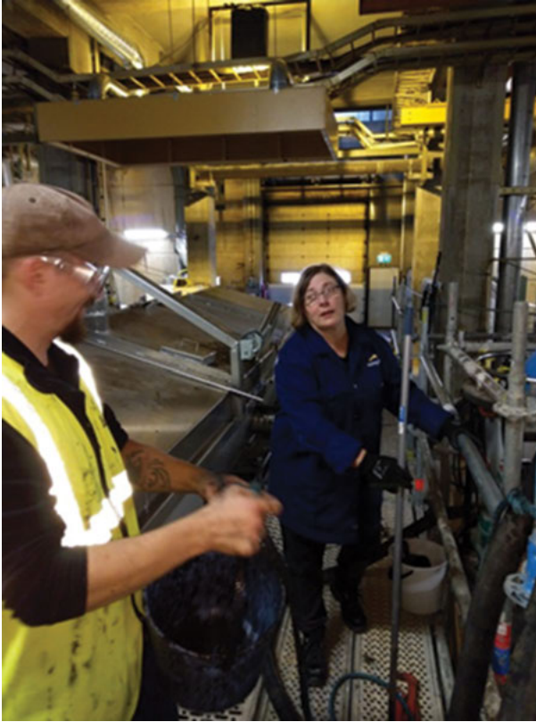
Figure 4.3: The zero fiber deposits from the lake bottom in Hiedanranta, Tampere, were processed in a bioreactor with approximately 15 \text{ m}^3 of effective volume. The exhaust gases were collected and measured. Maximal hydrogen concentration was about 4% in the emitted gas flow (containing the carrier gas). The lactate production rate was 9.2% (w/v). Photo: Elias Hakalehto.
