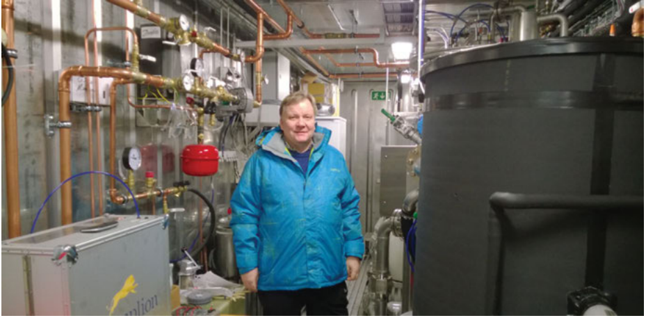
Figure 4.12: Elias Hakalehto, Adj. Prof., PhD, inside the ABOWE movable pilot plant in 2014. This biorefinery unit contained four tanks: 1. homogenizer, 2. hydrolyzer, 3. bioreactor (patented), and 4. product collection tank, as well as the computer (or satellite) control unit and a small laboratory. Photo: Ari Jääskeläinen. “Future biorefineries are industrial fields, where side streams from industries and municipalities are treated into useful products in successive process solutions. All waste is then integrated as a raw material into them” (statement by Elias Hakalehto, 2014).
