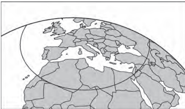
Figure 11.11 A generic footprint of EUTELSAT satellites. (Source: Colcy and Steinhäuser, 1993. The Third International Mobile Satellite Conference, Pasadena, California, 1993, co-sponsored by Communications Research Centre/Industry Canada and Jet Propulsion Laboratory/NASA.)
