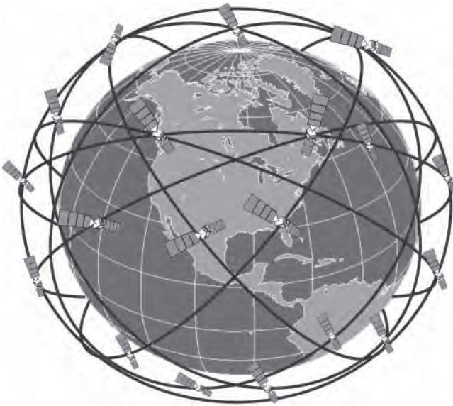
Figure 11.24 A schematic of the Globalstar constellation. (Source: Globalstar. Reproduced with permission of Globalstar.)
