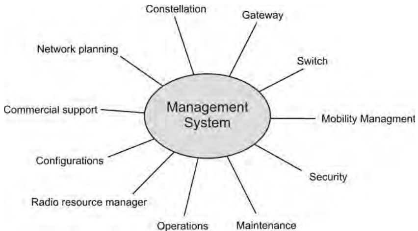
Figure 9.1 A telecommunications management network structure of a MSS
