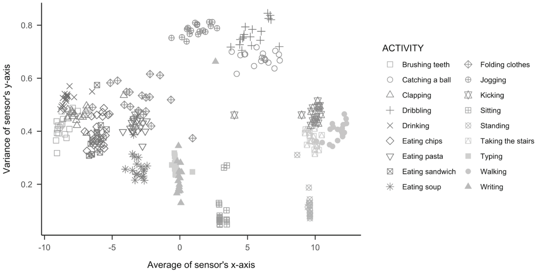
FIGURE 17.1. A two-dimensional feature space for activity classification. Observations of different activities (shown in different shapes) are plotted with the empirical average deflection measured on the x-axis of the accelerometer in a smartwatch (which partly reflects rotation of the arm in one axis) against the variance of activity on the y-axis (reflecting physical activity in one direction). A typical classification problem is to predict a person’s activity from such features. As can be seen, these two features alone are already quite informative for distinguishing various activities. This figure is available at https://github.com/brandmaier/mobile-sensing-figures under a CC-BY4.0 license.
