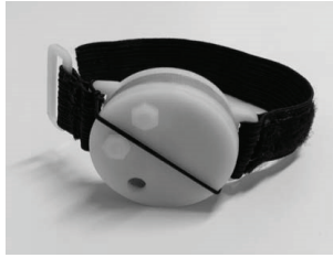
FIGURE 31.2. The EmotionCheck device, which can make users feel calmer using subtle haptic feedback. From Costa et al. (2016). Reprinted with permission from the Association for Computing Machinery.
