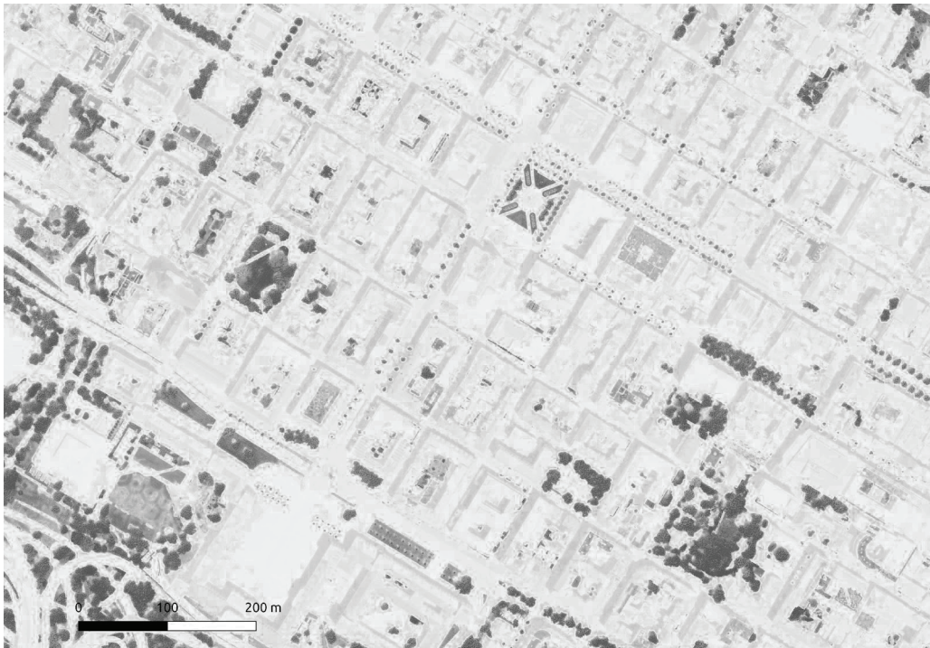
FIGURE 4.3. Example raster data. The maps show the amount of green present in the city center of Mannheim, Germany. The data are stored in a raster format. Each cell contains a value that represents the amount of vegetation (NDVI).
