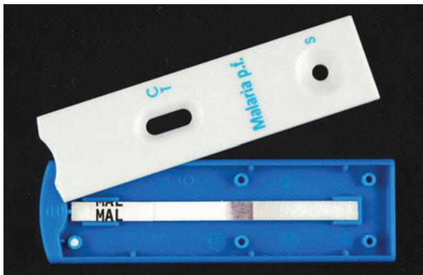
FIGURE 4 Inside view of a malaria RDT cassette showing the nitrocellulose strip with the specimen/buffer pad (left), conjugate pad (red because of the colloidal gold), and absorption pad (right). Note that the cassette has a single specimen (sample)/buffer well.
