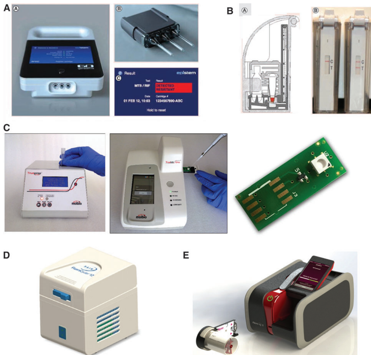
FIGURE 7 Selected NAAT platforms currently under evaluation or in development. (A) The Epistem Genedrive system for the detection of Mycobacterium tuberculosis , into which the cartridge with three ports that serve as reaction tubes are inserted. The results screen is also shown. (B) A schematic of the XCP Nucleic Acid Device (Ustar Biotechnologies), which is used in conjunction with the EasyNAT TB test (Ustar Biotechnologies) cartridge. The cartridge contains a plastic bulb with both the reaction mix and a lateral flow running buffer. This is inserted into the detection chamber holding the lateral flow test strip. After 5 to 10 minutes the result is read. Examples of negative and positive test results with control bands are shown. (C) The equipment made by the Molbio Group (India) required to process specimens and extract DNA (Trueprep) and monitor amplification (Truelab UNO real-time PCR analyzer) and the chip used for the detection of DNA. (D) The Fluorocycler (Hain Lifesciences) which is used for the semi-automated detection of TB using the Fluorotype MTB test. (E) The Aleris Q system and cartridge, which are currently being developed for the detection of TB. It performs on-board sample processing, lysis, DNA extraction, and TB detection. Sputum is collected in a special container that is attached to the test cartridge, which is then inserted into the machine. A and B are republished with permission from reference 138. C, D, and E are republished with permission from reference 37.
