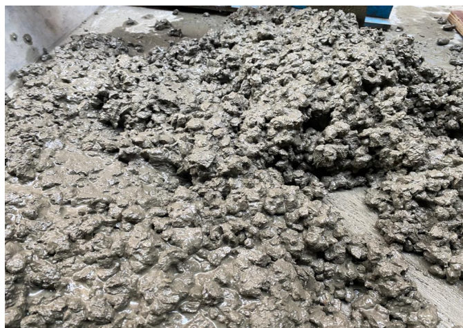
FIGURE 3.3: Concrete mix containing 15% waste PET bottle particles and steel fibers
