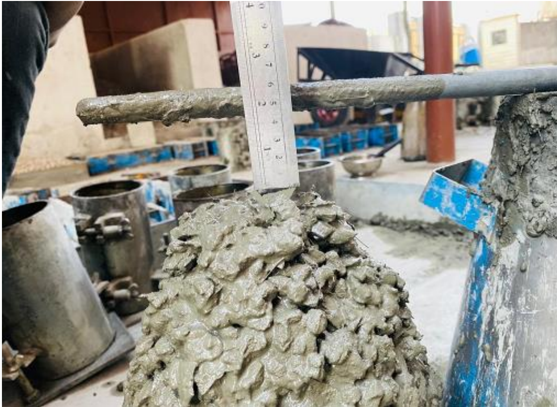
FIGURE 3.4: Slump of concrete having 15% waste washed PET bottle particles and steel fibers
