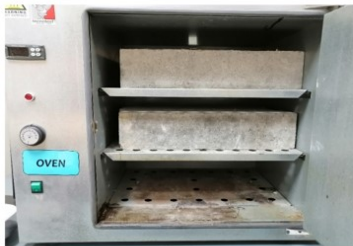
FIGURE 3.4: Drying Samples in Oven for Water Absorption and Mass Loss Test
