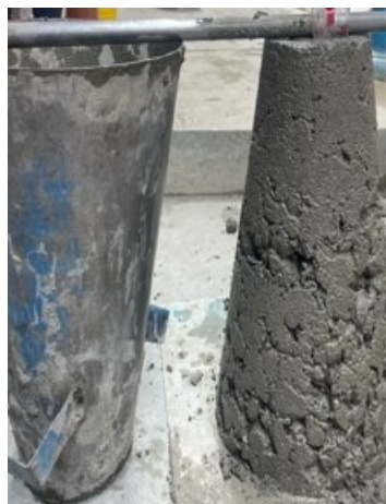
FIGURE 4.1: Measuring Value of Slump of PNMDPESP-FRC
