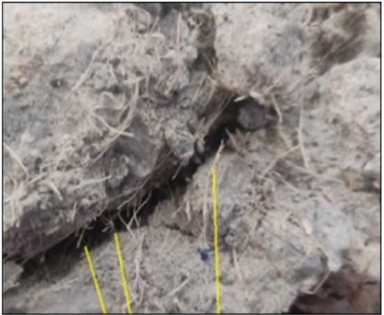
Breakage of banana fibers
