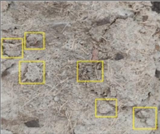
Sticked small particles due to fibers
