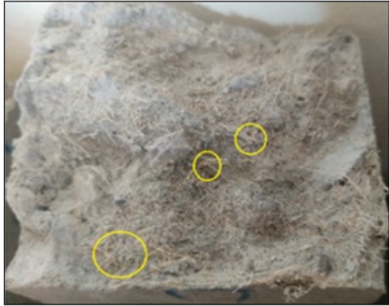
Bond of fibers with surrounding matrix
