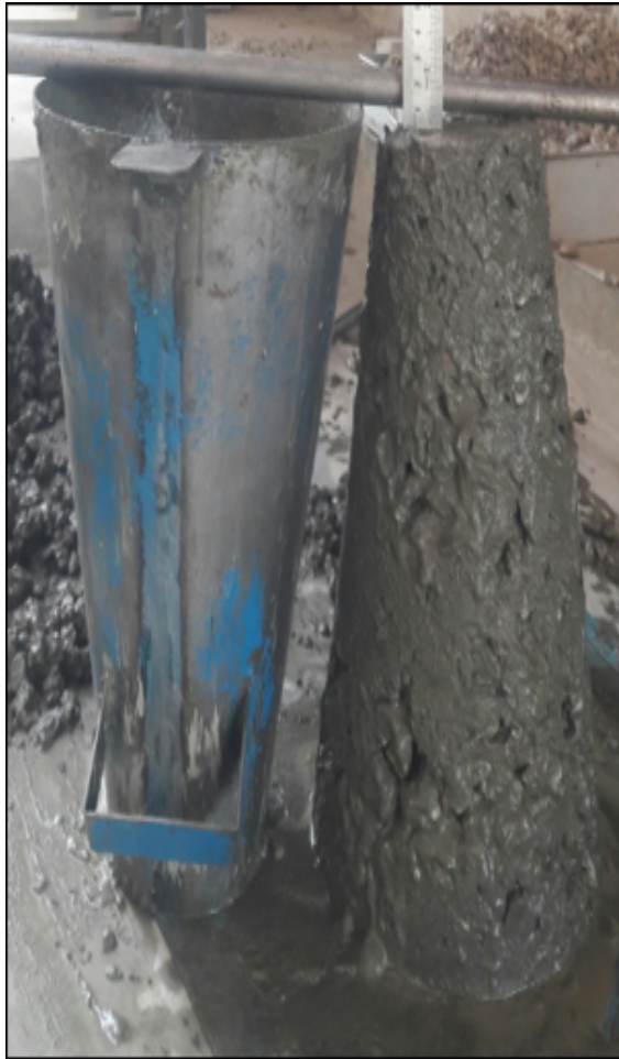
FIGURE 3.1: a) Measuring the Value of Slump of UBFR, b) Combined effect of UPEO and BF on the relation between slump of fresh concrete and density of hard concrete
