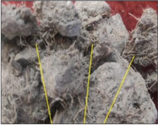
Bridging effect of fibers
