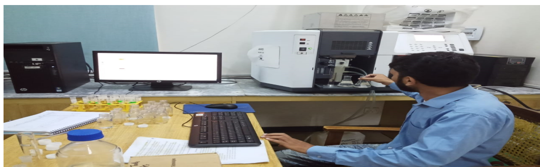
FIGURE 3.2: Zinc analysis with the help of Atomic absorption spectrophotometer
