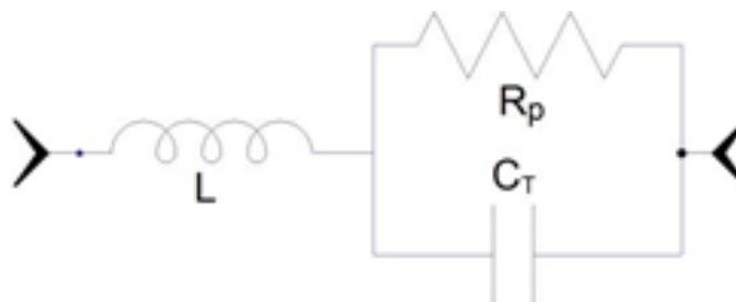
FIGURE 2.4: Model of lumped element components in reverse biased condition
