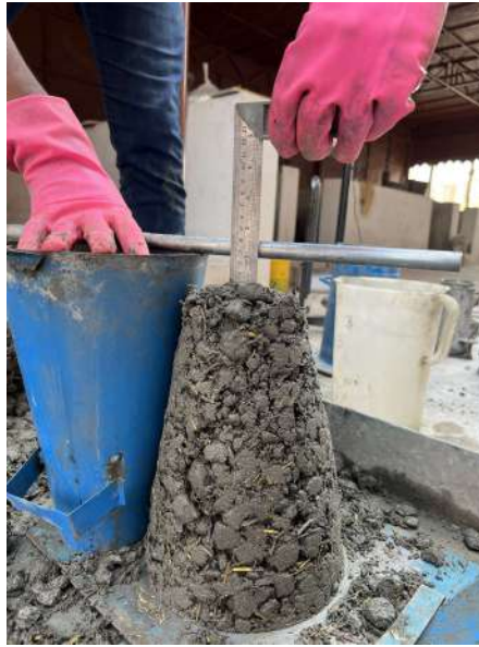
FIGURE 4.1: Slump Test of WSRC
