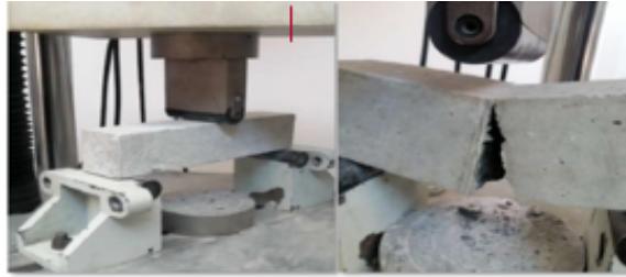
FIGURE 4.3: Flexural Strength Testing
