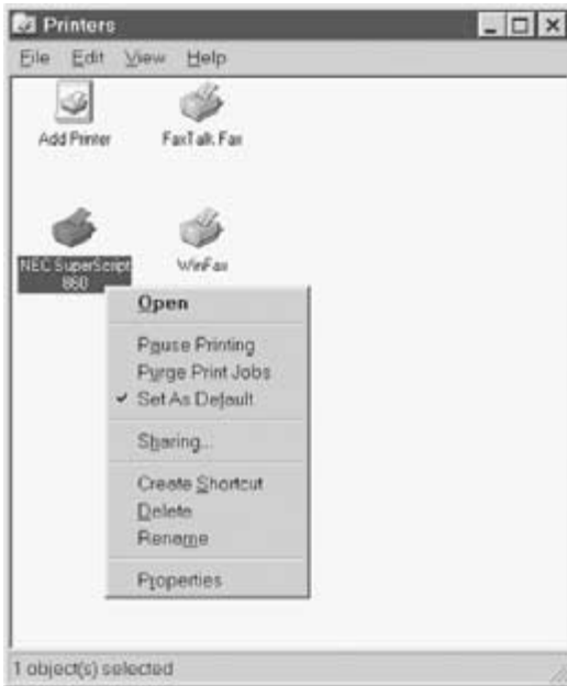
Figure P-4 A printer can be configured as the default printer and for sharing by other computers on the network.
