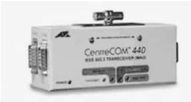
Figure T-6 This four-port transceiver from Allied Telesyn has a BNC connector ( top ) that is used for connecting the unit to a 10Base2 (thin coax) Ethernet LAN.
