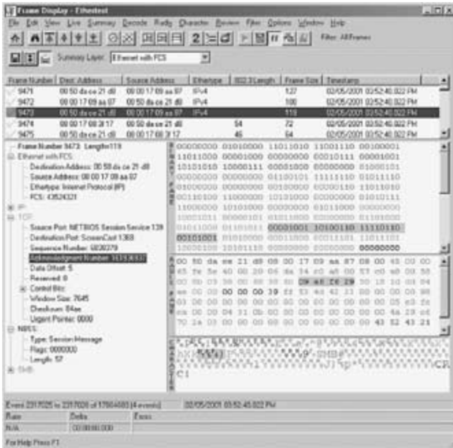
Figure P-8 Frontline Test Equipment offers a protocol analyzer called Ethertest that runs on Windows platforms. The “Frame Decode” pane of Ethertest’s Frame Display window provides a comprehensive layered decode of each frame/packet, allowing a problem to be quickly located. Protocol errors are highlighted in red, making them easy to recognize.
