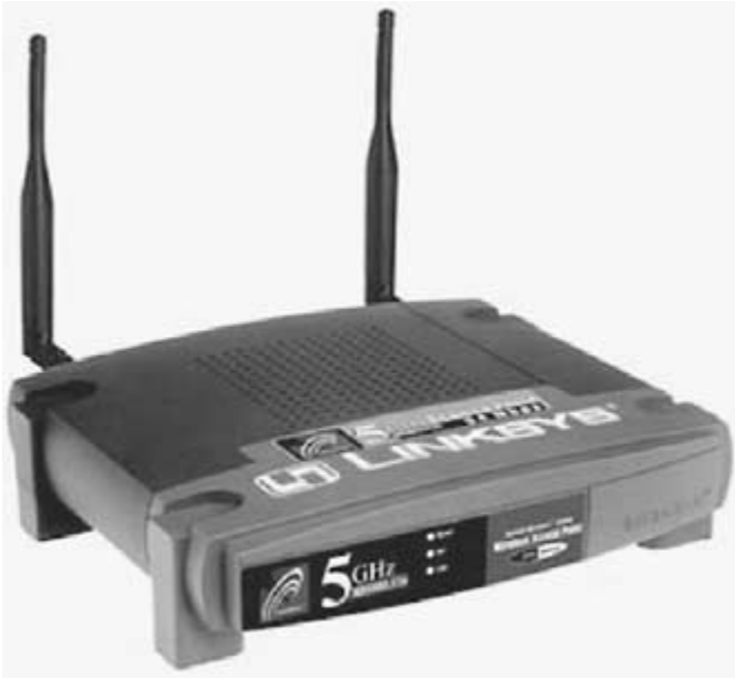
Figure A-3 An example of a consumer AP is this 5-GHz Wireless AP (WAP54A) from Linksys, which features antenna with a range of up to 328 feet indoors.
