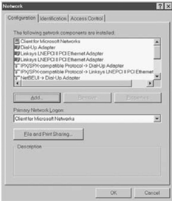
Figure P-1 To verify that the right drivers have been installed, the user opens the Network Control Panel to check the list of installed components. In this case, a Linksys LNEPCI II Ethernet adapter has been installed.
