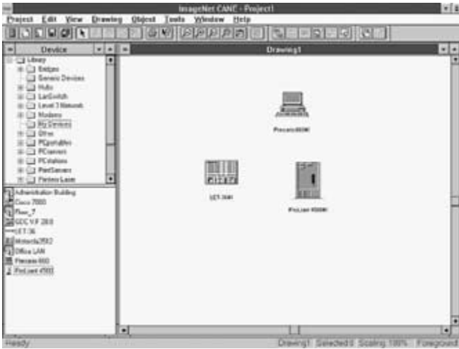
Figure N-1 Typically, a design tool provides workspace into which objects are dragged and dropped from device libraries to start the network design process from scratch. (Source: Netformx.)
