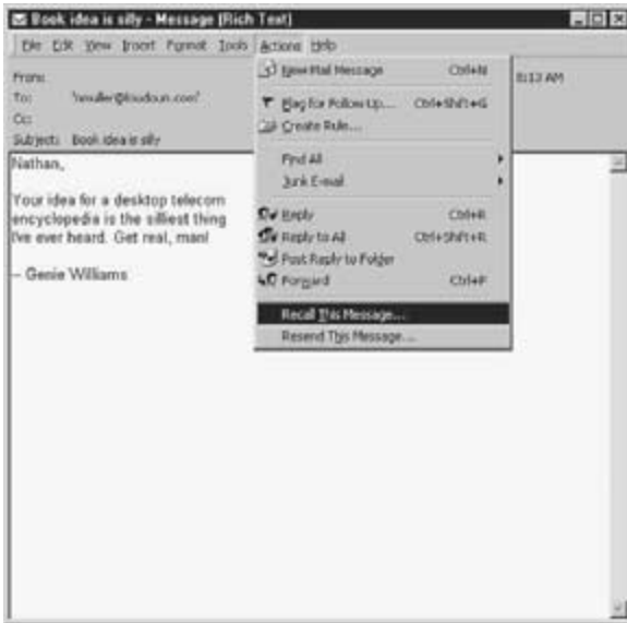
Figure E-3 When Microsoft Outlook is configured as an IMAP client, it can recall or replace a sent message, provided that the recipient has not yet opened it.
