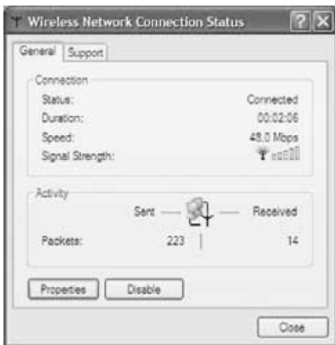
Figure A-2 The 5-GHz DWL-5000 AP from D-Link Systems, Inc., keeps the client device notified of the status of the wireless link. In this case, the signal is at maximum strength and is capable of a data transfer rate of 48 Mbps.
