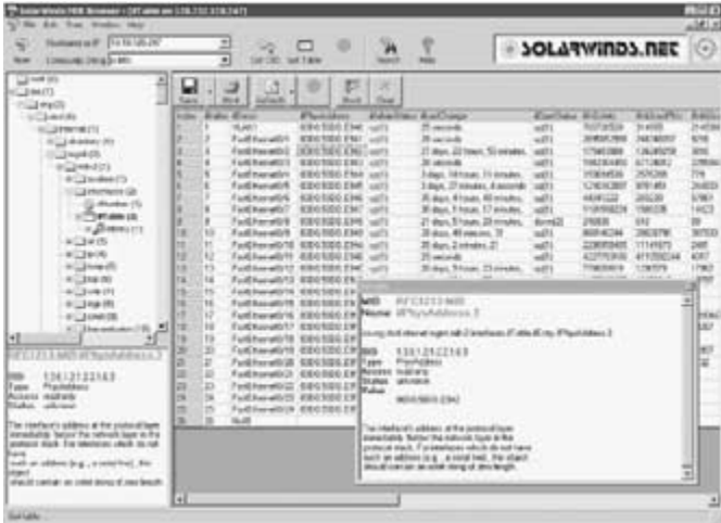
Figure S-3 The MIB browser from SolarWinds.Net, Inc., is capable of reading over a thousand standard and proprietary MIBs and 110,000 unique OIDs.
