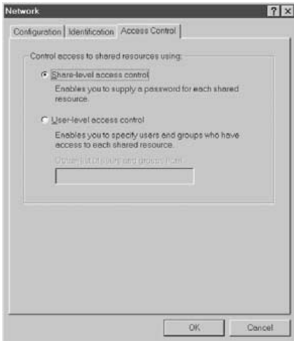
Figure P-3 Choosing share-level access allows the user to password-protect each shared resource.
