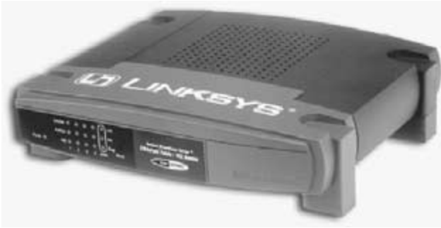
Figure R-5 The Linksys Instant Broadband EtherFast cable/DSL router is representative of the new breed of user-friendly multifunction routers aimed at the emerging home networking market.
