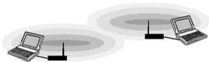
Figure W-1 A wireless peer-to-peer network created between two notebook computers equipped with external wireless adapters.
