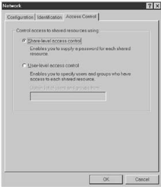
Figure H-7 Choosing share-level access allows the user to password-protect each shared resource.
