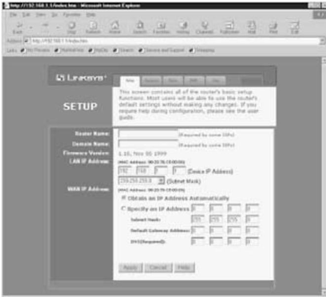
Figure D-4 The Linksys Instant Broadband EtherFast Cable/DSL Router is one of a growing number of off-the-shelf products that is easily configured by the user through a Web browser interface.
