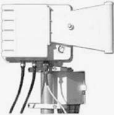
Figure L-6 A multisector antenna at the carrier's hub location transmits/receives traffic between the antennas at each customer location.
