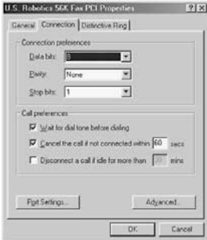
Figure A-9 The connection preferences for a U.S. Robotics 56-kbps fax PCI modem as configured from within Windows 98.
