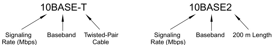
FIGURE 8.2 Baseband and broadband IEEE 802.3 LANs are designated by bandwidth in Mbps followed by either the type of cable it supports or its maximum length in meters.
