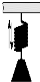
FIGURE 4.2 An object is attached to a spring that is suspended from a ceiling. When pulled and released, the spring oscillates up and down. This oscillation is called simple harmonic.
