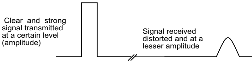
FIGURE 4.15 The combined effects of capacitance and attenuation result in a signal that is received distorted and weaker than what it was when transmitted. This can severely impact the performance of a network. Source: Adapted from Leeds & Chorey, 1991a.
