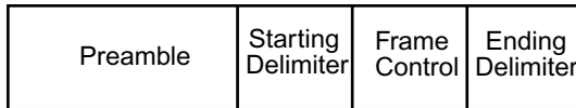
FIGURE 10.4 FDDI token format. The preamble consists of 16 or more I symbols; the starting delimiter consists of one JK symbol pair; the frame control consists of two symbols; and the ending delimiter consists of two T symbols.
