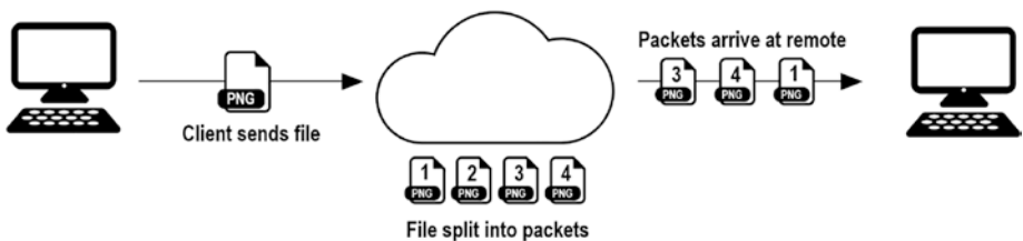
Figure 1-3. File split into smaller packets, packet loss and packets received out of sequence
