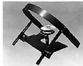
Figure 4.7 A pyranometer with shadow band (Courtesy: Eppley Laboratory)
