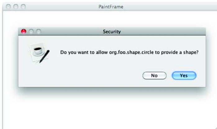
Figure 14.3 Secured paint program prompting the user to grant the unsigned circle bundle permission to provide a shape service
