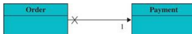
FIGURE 9.23 How the original visibility of Figure 9.22 must be considered for a specific instance if a contract has a more restrictive precondition.
