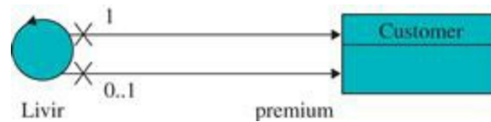
FIGURE E13.11 A mandatory and an optional association to a façade controller.
