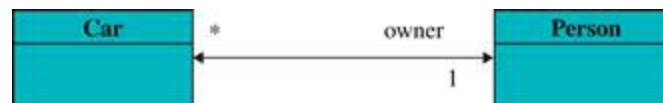
FIGURE E10.10 A bidirectional association with one mandatory role that can be updated.
