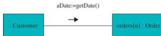
FIGURE 9.9 Communication diagram with a message being sent to the last element of an ordered set.
