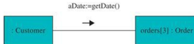
FIGURE 9.8 Communication diagram with a message being sent to a specific element of an ordered set.
