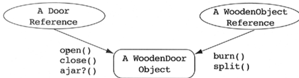
Figure 6.4. Multiple referencing of multiply derived objects.
