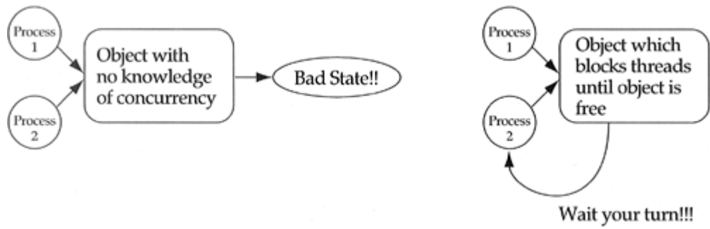
Figure 9.14. Example of an active object.
