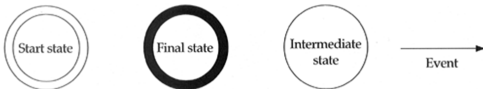
Figure 2.8. State-transition diagram notation.
