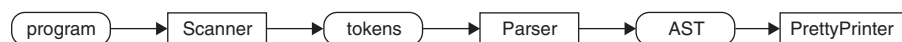
FIGURE 9.5 The phases of manipulating a program. The rounded items are the data and the rectangular items are the manipulators.
