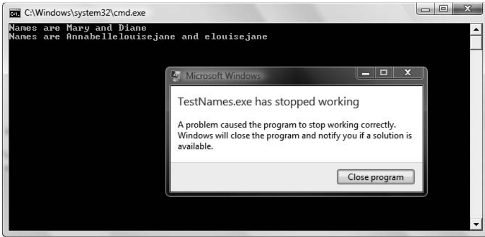
Figure 5-39 Output of the program in Figure 5-35 after “Annabellelouisejane” is assigned in strcpy()
