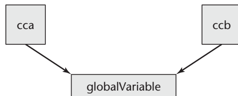
Figure 7.9 An example of common coupling.
