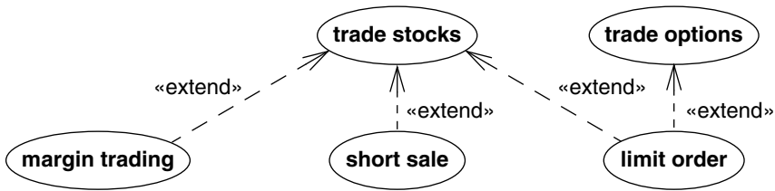
Figure 8.2 Use case extension. The extend relationship is like an include relationship looked at from the opposite direction. The extension adds itself to the base.
